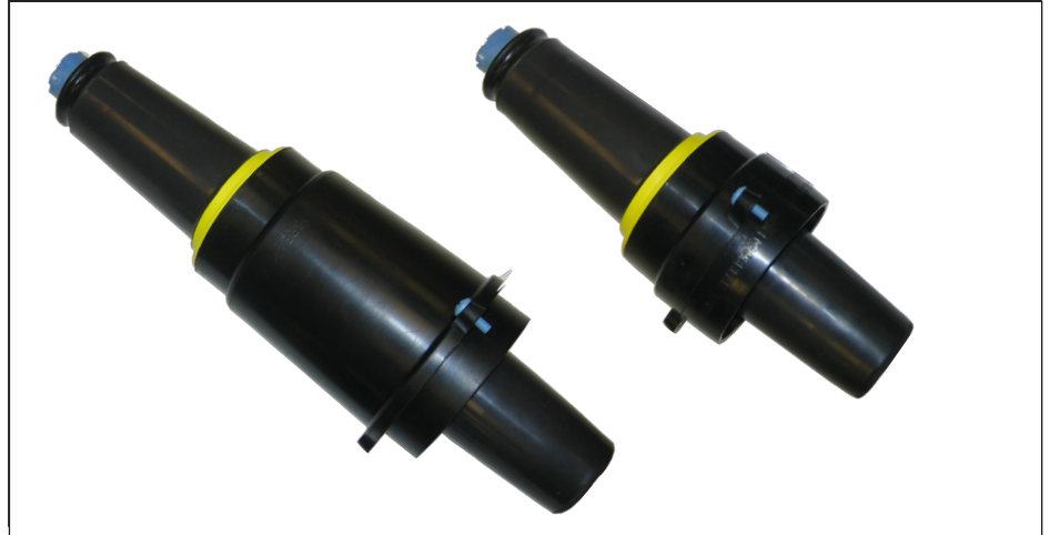
Figure 1. 25 kV Loadbreak Bushing Insert with latch indicator for applications in transformers, switches, and other apparatus (right). Longer version for use whenever increased clearance from the equipment faceplate and underground cables are required (left).
