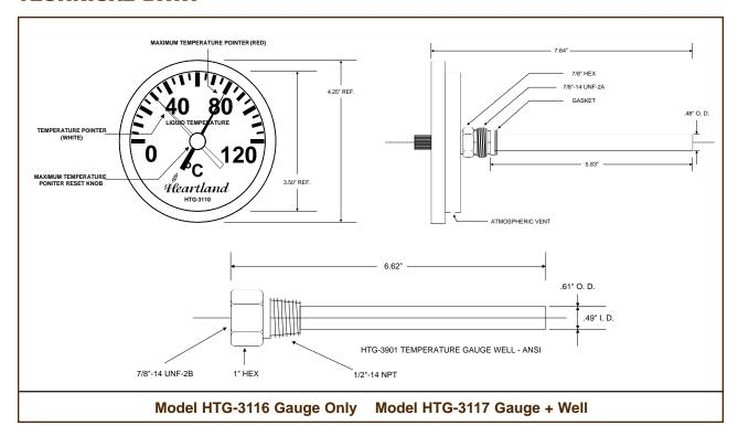
**OPERATION** Install Model HTG-3901 well in the transformer tank. Then, install the HTG-3116 temperature gauge into the well. The union connection on the gauge allows easy gauge centering. The temperature gauge is now ready to measure and indicate temperatures between 0 - 120 degrees centigrade.
