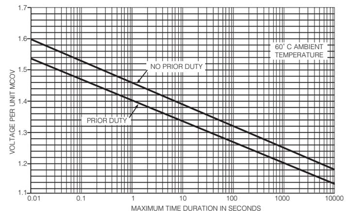
Note: The 24 hour TOV with prior duty is 1.07 per unit of  $U_C$ .
