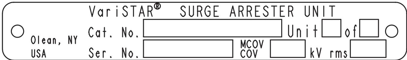
Figure 6. Detail of unit nameplate on arrester base.
