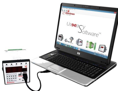
USB INPUT FOR PARAMETERIZATION THROUGH UseEasy™ software
