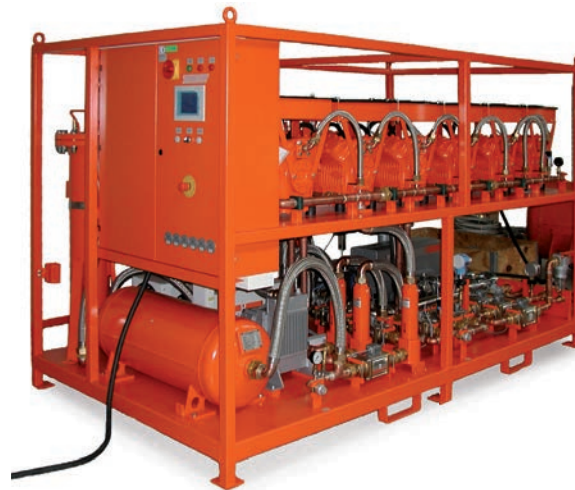
SF 6 gas handling plant for an electron accelerator
