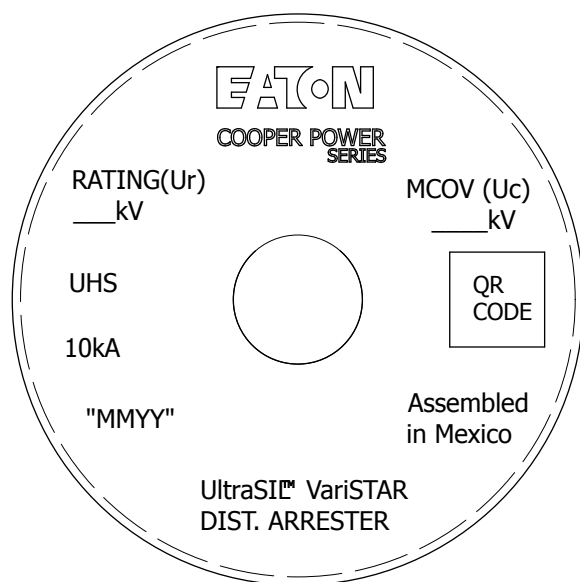
Figure 14. I_n = 10 kA, Class DH, UHS nameplate—stamped in stainless steel top cap
